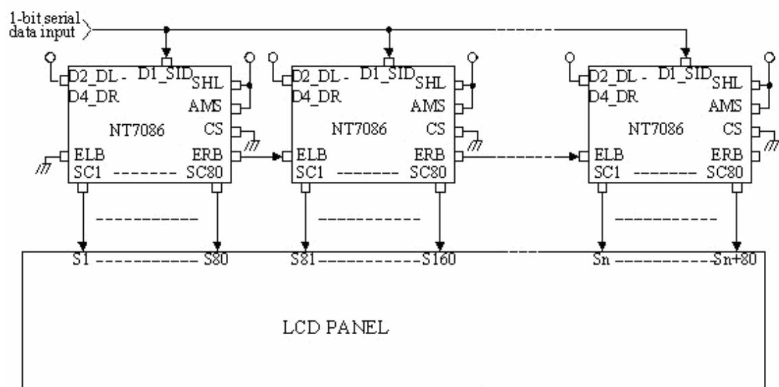
**4-bit parallel interface mode (80 Ch. Segment driver)**
