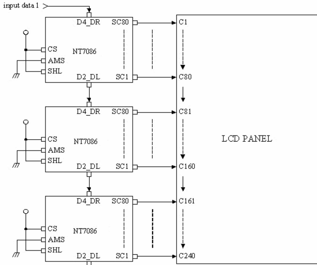
**Dual-type interface mode (40 Ch. + 40Ch. Common driver)**
