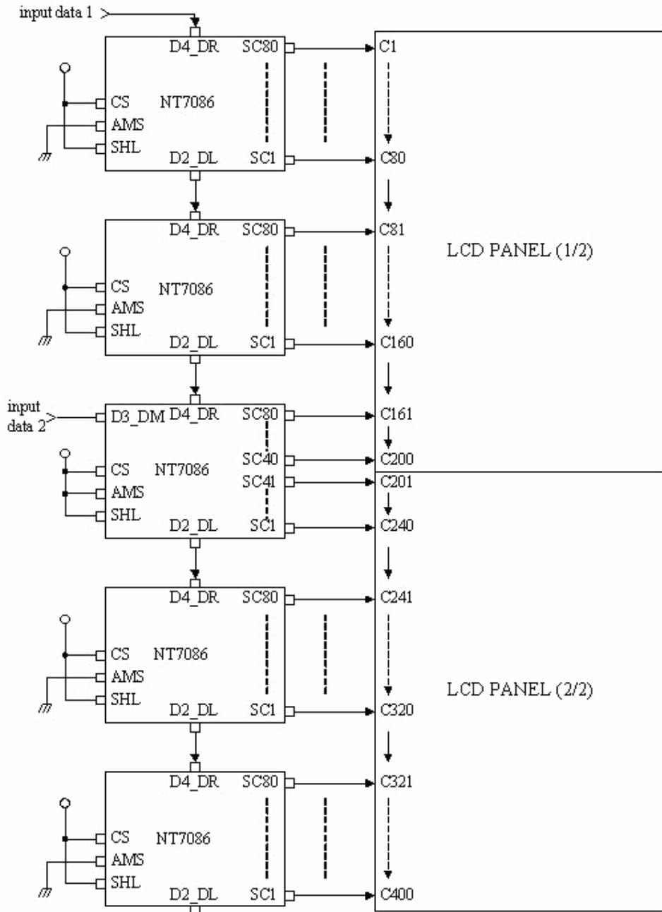
**NOTE:** Using this application mode (dual-type common mode), the duty ratio can be reduced to half. In case, 1/200 duty can be used to drive the 400 common LCD panel.
